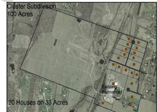
Above (top to bottom): The above illustrates how a conservation subdivision can be used to retain large tracts of farmland. The top illustration shows a conventional subdivision of 100 acres into 20 five-acre lots where the community’s zoning requires a minimum lot size of five acres per lot. The illustration below it shows a conservation (cluster) subdivision where the 20 building lots are clustered on 33 acres of the site – leaving 67 acres of prime farmland within a conservation easement. The conservation easement can be held by a homeowners association, land trust, or sold to an adjacent farmer for the agricultural value of the property that is far lower than the use value if it could be developed.
